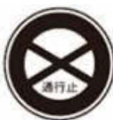
Road Closed 通行止め
